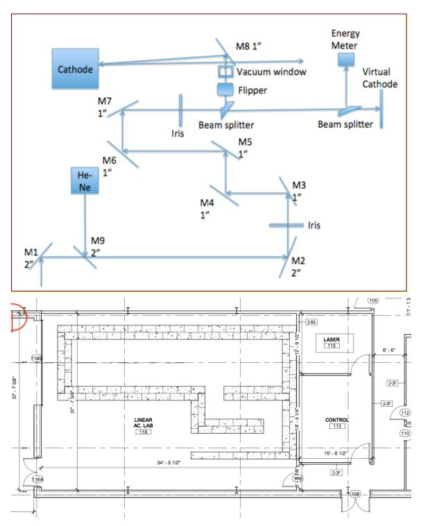
The entire laser transport line includes a laser control room, a laser room, and the laser line transport room. The laser transport line would be equipped with an iris, mirrors, and lenses in order to maneuver the laser beam in a way that the beam quality and size would be maintained, while still fitting in the predetermined 10m space. The positions of
